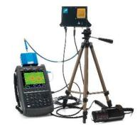
transmissions of 5G NR FR1 and FR2 control channels. Provides key performance indicators including physical cell ID, received power levels and beam index information. Conducted EVM measurement is also included with Option 37
